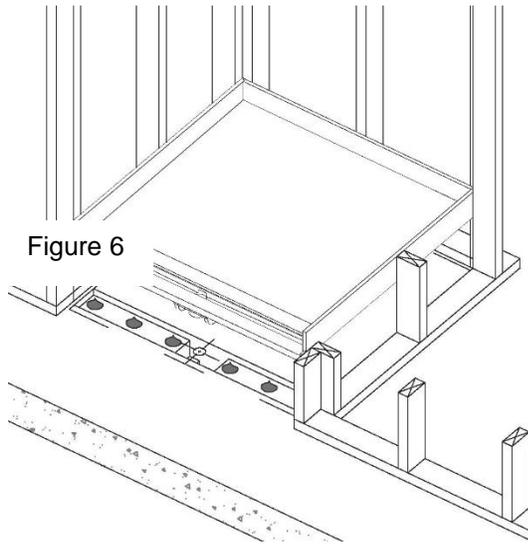
Remove the base from the dry fitting step. Clean and vacuum trench and shower base floor install area.
